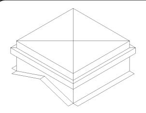
The Universal Cupola Base is designed with the installer in mind. Factory prepped at 4-12 pitch, this cupola base is factory assembled and requires no wood curb. It will adapt to roof pitches between 1-12 & 7-12. The same unit can be utilized for vented and non-vented applications. It is ideal for new construction or retrofits, as it can be installed on top of purlins or steel roofing. The Universal Base is available with a universal trim kit or powder coat option.
