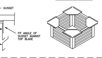
TO INSURE A STRUCTURALLY SOUND PRODUCT, WE INCLUDE (4) GUSSET PLATES WITH THE 36" AND 48" ROOF SECTIONS. EACH GUSSET HAS "VHB" TAPE ON THE BOTTOM SIDE. REMOVE THE FILM FROM TAPE AND POSITION GUSSET IN EACH CORNER OF SIDE ASSEMBLY AS SHOWN. APPLY PRESSURE TO THE TOP SIDE OF EACH GUSSET SO TAPE CAN ADHERE TO SIDE SECTION. TAPE WILL ADHERE IN APPROX. 5 MIN. DURING ASSEMBLY.
